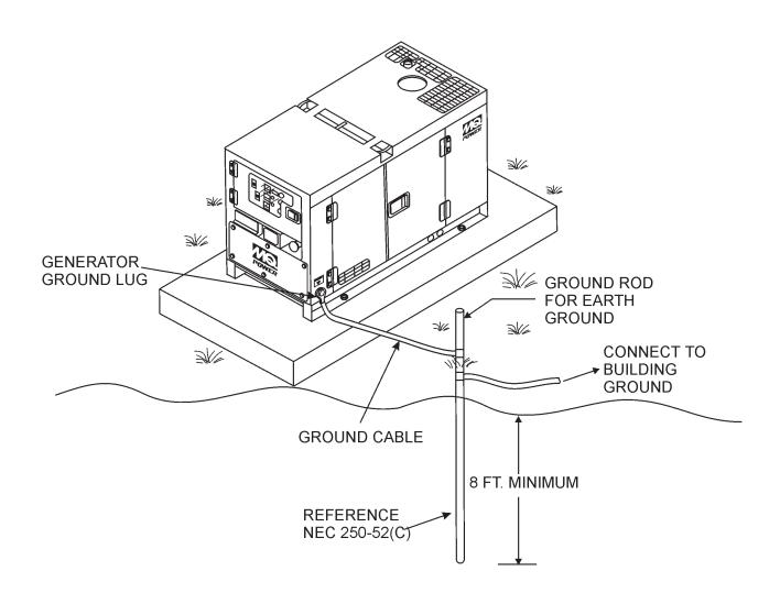
Figure 3. Typical Generator Grounding Application
